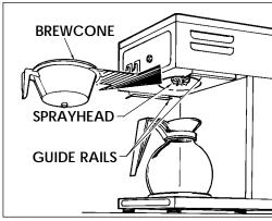
Figure 1. Sprayhead and brewcone rails.
