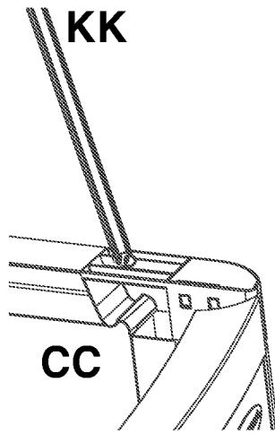
**18.** Rotate the Lid Support Prop Rod (KK) so that the small cylinder end will pass through slot in the top front of Upper Side Panel (CC or EE as Prop Rod can be placed on either right or left side).
