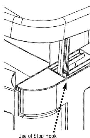
**21.** To open the Lid to the 6 inch position, lift Lid up past 6 inches, pull Prop Rod towards outside of Upper Side Panel, and lower lid until the stop hook engages with the side panel. This allows front doors to be opened without lifting Lid all of the way.
