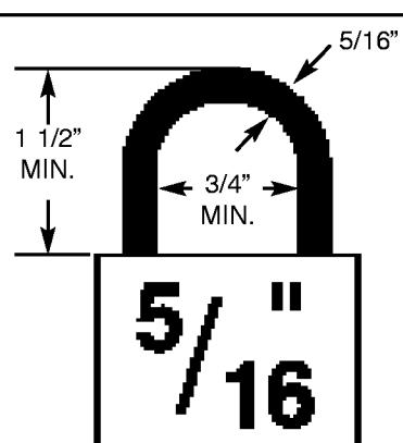
**Securing Your Shed:** To properly lock your shed using the Padlock Assembly feature, 5/16" padlock is recommended.
