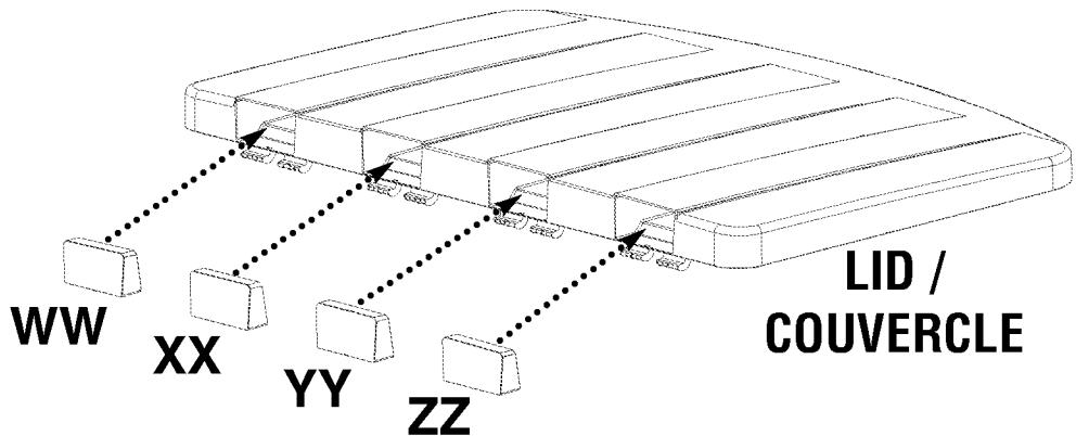
**20.** Hold Lid in an up / open position parallel with the Upper Back (DD) then hook the Lid hinges to the Upper Back hinge receptacles. Carefully close Lid to engage.
