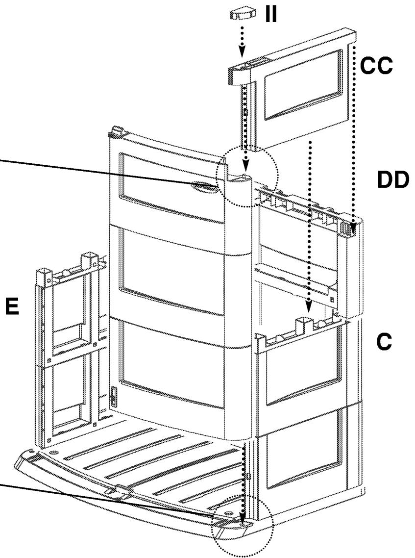
**14.** Place Upper Right Side Cap (II) in upper right side cap receptacle located in the Upper Right Side Panel (CC). Press down until Upper Right Side Cap snaps into place.
