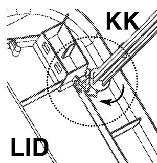
**19.** Locate the cylinder receptacle on the underside of the Lid at the front right or left corner.
