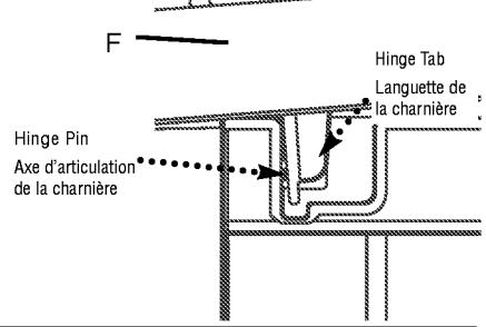
6. While bending the other hinge tab slightly towards the middle of the seat, push down firmly on the Lid until the hole in the hinge tab engages with the hinge pin.
