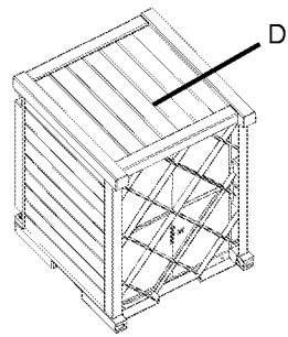
5. Working from the back of the unit, position Lid F in the closed position as shown. Slide the Lid sideways so that one hinge hole in the hinge tab engages with hinge pin on the Back Panel.
