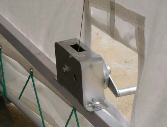
Winch Assembly Mounted To Lower Front Panel Beam
