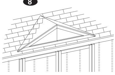
8-9. If building is not shingled, shingle roof first. Follow all manufacturers instructions for shingling. Overlap reverse gable by 6" or more as shown in figure 8. If a shingle does not run up gable by 6" cut tab off and run a full shingle up gable. Once roof is completed then shingle reverse gable as shown in figure 9. Run reverse gable shingles all the way to the valley where the roofs meet. Cut the shingles on the reverse gable back by 2".
