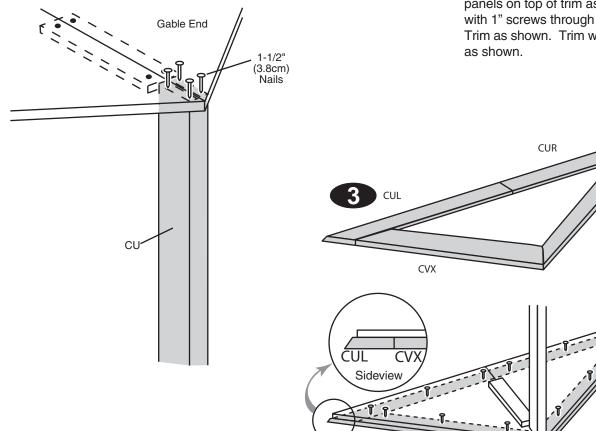
(12)-1"(2.5cm) Screws  Position second Large Roof Panel flush to first Panel and Trim. Secure with four 1-1/2" nails into Trim CVX and with two 1-1/2" nails into Ridge Board CU.
