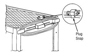
For safety and neat appearance, secure cord plug to cord with plug snap.
