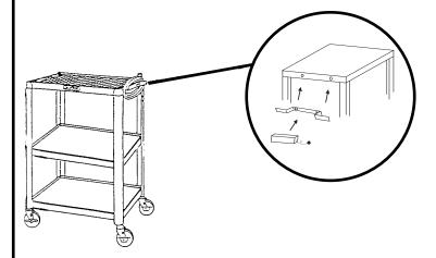
Place metal cordwrap onto metal top shelf making sure that the holes on the cordwrap align with the holes on the shelf. Place the two screws through the holes of the electrical assembly. Place the electrical assebly with the two screws through the holes of the cordwrap and mounting bracket. Secure screws with wingnuts.
