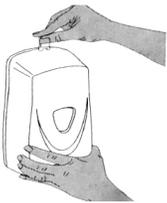
To open the dispenser cover, insert key into slots at the top of the dispenser. Dispenser will automatically shut off when cover is opened.
