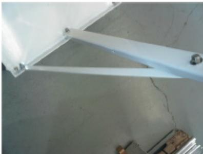
6. Tighten all nuts and bolts to ensure rigidity of the floor stand.
