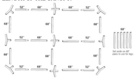
2. START FROM THE CENTER AND COMPLETE THE CENTER FRAME. THEN ASSEMBLE EACH SIDE.
