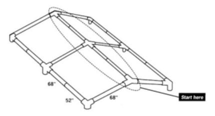
3. PLACE TARP OVER FRAME. TIE BUNGEES AS SHOWN IN DIAGRAM. WHEN TYING BUNGEES, ALTERNATE FROM ONE SIDE TO THE OTHER FOR EASIER INSTALLATION.
