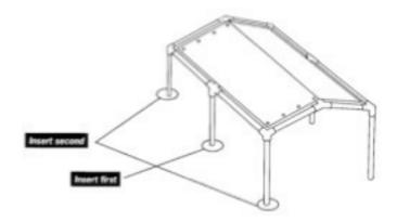
NOTE: FOR MORE PERMANENT INSTALLATION ANCHOR FRAMEWORK TO GROUND USING TIE DOWNS OR THE PROPER ANCHOR KIT FOR YOUR NEEDS.
