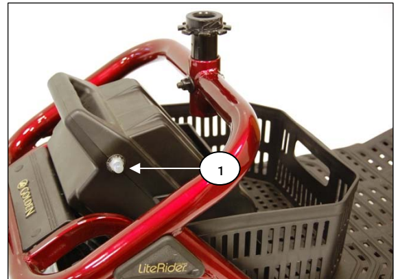
Figure 27. Main Circuit Breaker
