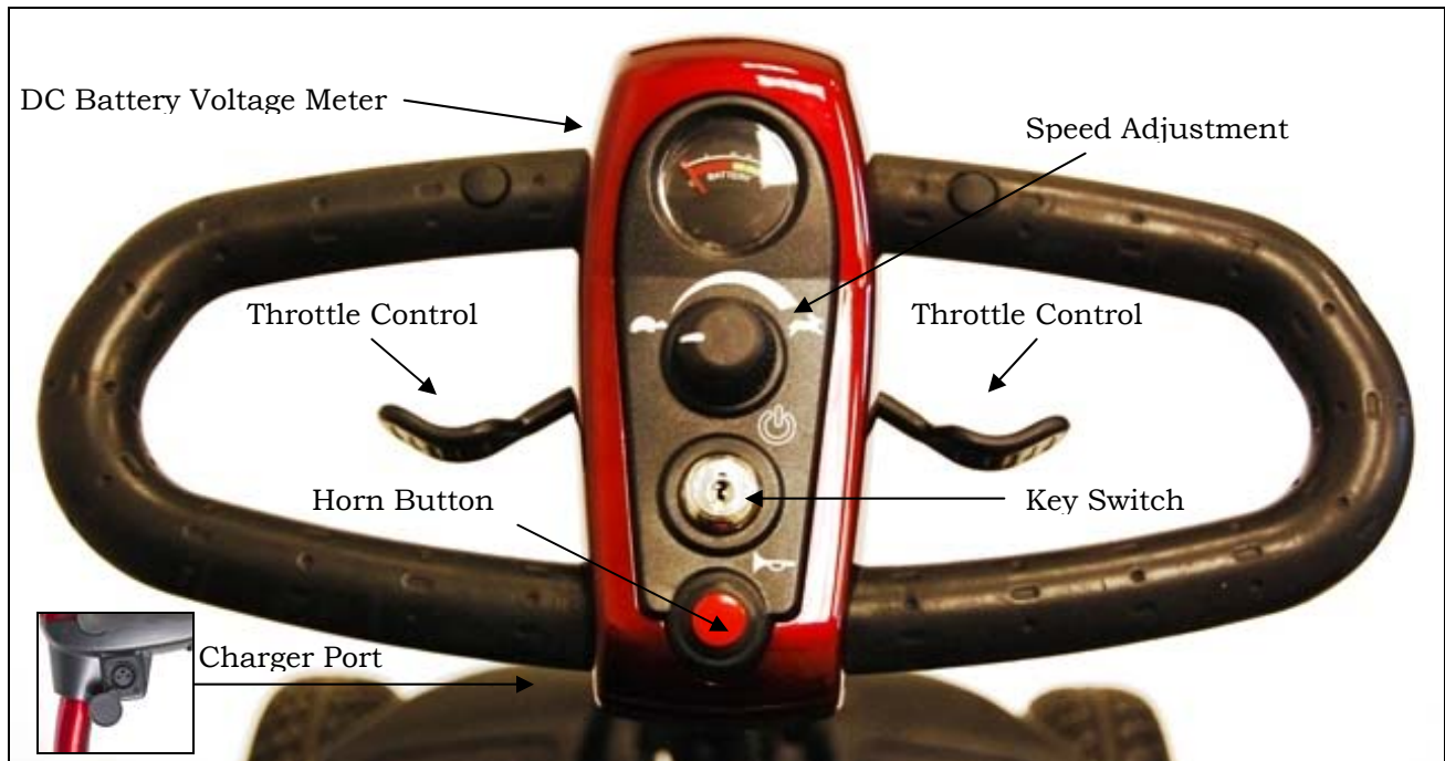
Figure 5. LiteRider™ Delta Tiller Control Panel
